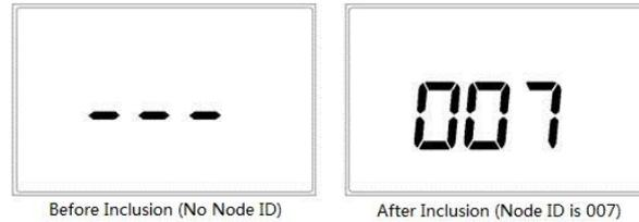
After inclusion, turn off the device and then turn it on. Now the device is ready to be operated by controller/ gateway in Z-Wave network.
